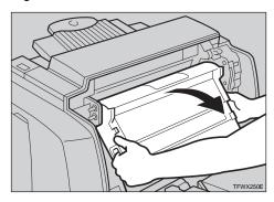
Holding the green inset grips of the photoconductor unit, remove the unit from the printer, and place it carefully inside the new photoconductor unit's box.
